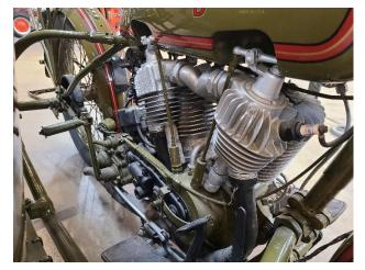
The 74 cubic inch 9.45 horsepower V-Twin with Schebler carburetor found on the 1925 JD is an F-head, or Intake Over Exhaust (IOE) model, a four-stroke engine whose valvetrain comprises Overhead Valve (OHV) inlet valves within the cylinder head, and
