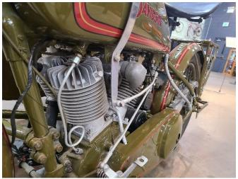
stroke, "wasting a spark." The exhaust note is a signature throaty growl with occasional popping. Thus the design of the engine creates a plug firing sequence that is the origin of the engine's unique sound.
