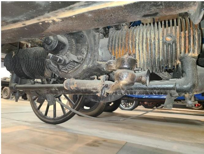
of the vehicle was the gas tank, not a radiator, as the air-cooled engine didn't require a water reserve. With an estimated top speed around 15 miles per hour, the Model A was built for rugged dependability more than speed.
