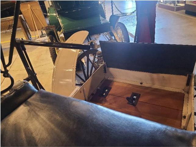
Steered with a tiller, the vehicle had a tiller-mounted throttle and a shift lever on the driver's left hand, with two pedals on the floorboard: a "clutch" and a brake. Although unconventional by modern standards, this era saw constant experimentation in controls, and this arrangement would not have stood out as unusual at the time.
