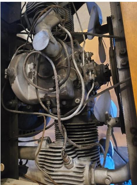
This vehicle has an air-cooled, horizontally opposed, two-cylinder engine. Located under the floorboards beneath the driver's feet, the engine was crank-started in the front. This model was rated at 10 horsepower, with a top speed around 25 mph, but later models sported an improved 14 horsepower engine.
