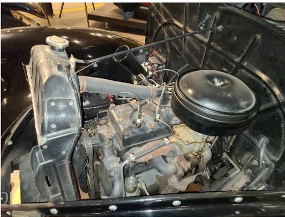
The 134.2 cubic inch engine is an inline L-head 4-cylinder, with a one-barrel Tillotson carburetor, providing about 48 horsepower. Despite the lower horsepower, the smaller-bodied Willys models of this time were still known for producing decent speeds with good fuel economy. Their light-bodies also made them popular with hot-rodders of the era. The transmission is a 3-speed floor-shift manual. This model came equipped with four-wheel mechanical brakes and steel disc wheels.
