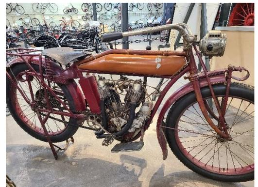
This 1913 bike utilizes a magneto ignition with a pedal crank start. Indian experimented in 1914 with an all-electric starter, but discontinued after one year due to deficiencies in existing storage battery design. 1913 was one of the last years to feature a pedal-crank start, pedals were all but gone by the introduction of the Powerplus model in 1916.
