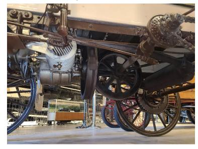
roller to break contact from the flywheel putting the car in "neutral" so it could be cranked without rolling forward.
