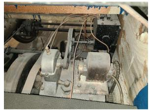
two-cylinder engine, producing about 16 horsepower. A friction-transmission with two forward speeds and one reverse transferred power to the chain-drive system to the wagon-style, solid-rubber shod wheels on either side in the back. The tank on the front
