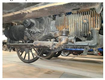
of the vehicle was the gas tank, not a radiator, as the air-cooled engine didn't require a water reserve. With an estimated top speed around 15 miles per hour, the Model A was built for rugged dependability more than speed.
