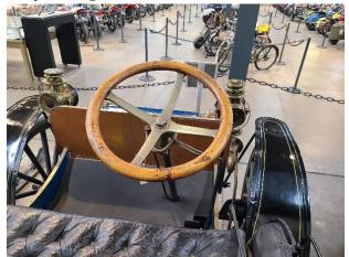
body. IHC's first true truck, the Auto Wagon was designated the Model A from 1908 until 1911, and Auto Wagon sales in 1909 led the emerging light truck market. Despite the designation, the Auto Wagon was built on the same chassis as the Buggy, and the Wagon bench seat and tray could be put straight onto an Auto Buggy chassis.
